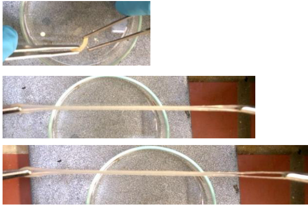
1% CNC as prepared, tensile trial
